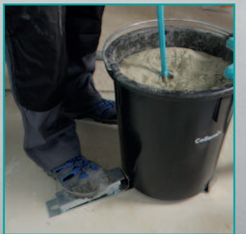
A full body system, which fixes the bucket in place ergonomically and without strain.
