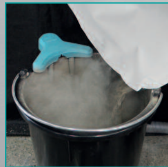
The dust.EX extracts the material directly from the bucket — almost no dust escapes.
